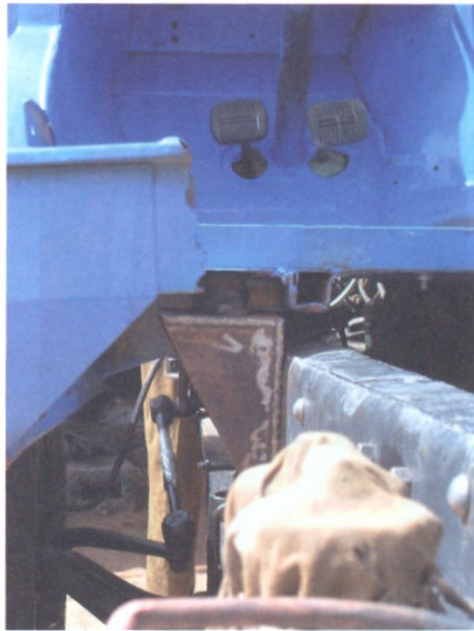
Photo 6.7 Reinforcing the cabin Source: K. Beck
